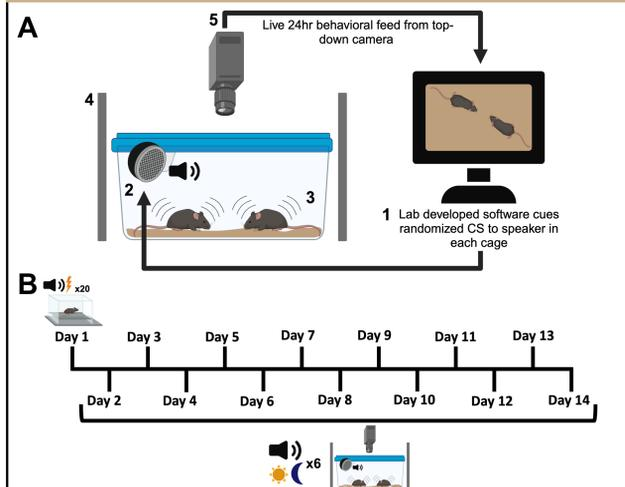
**Fig 1. A novel method for assessing CS conditioned fear in the home cage.** A. Integration of software and behavioral recording. 1. The software triggers the CS. 2. CS are played through speakers in each cage of 3. group-housed mice. 4. Each cage has sound-attenuating panels to control volume. 5. Top-down cameras record throughout light and dark cycle. C. Behavioral protocol for fear conditioning and home cage CS delivery across day/night.
